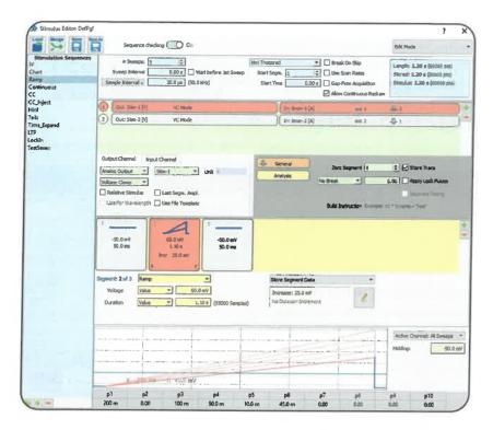
In this editor you define the pattern of the stimulation sequence. You have access to all output and input channels of the EPC 10 USB amplifier. Numerous different segment classes, an Increment Editor and a File Template Editor allows you to create almost every possible stimulation sequence.
