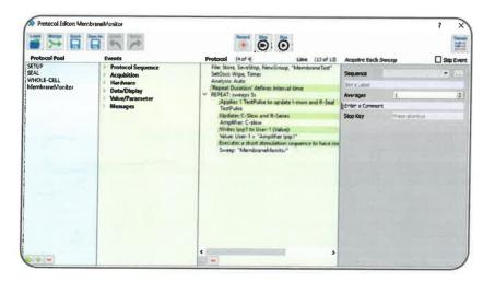
The Protocol Editor allows to create experimental protocols via an event list which is processed in the given order. In addition to data acquisition one can now control or interact with external devices, react to analysis results or create conditional loops including break conditions or assigned keys. The predefined protocol lines allow a highly standardized and automated experimental procedure.
