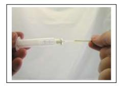
Micromanifolds<sup>®</sup> can be stored wet or dry. If calcium builds up internally, flush with vinegar for at least 1 hour and then distilled water. Micromanifolds can also be sonicated.
