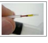
Remove the Micro valve from the quartz capillary, and using a syringe with a 1mm ID length of silicone tubing, inject water into the valve. About 1ml is all that is needed to flush out the valve. After flushing you can test the Micro valve by pulling back on the syringe. If the valve is working, the plunger will not remain extended after letting go.
