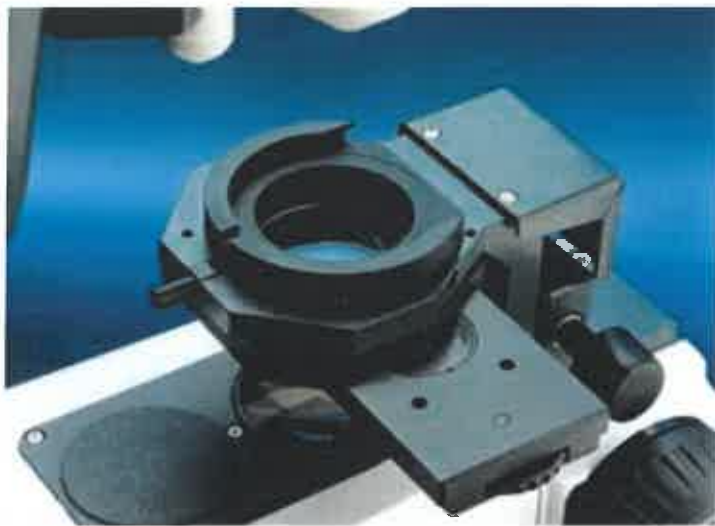
The polarizer slider has two positions, one for visible and one for infrared light. The contrast adjustment according to Sénarmont is performed by turning a knob to the right or left.
