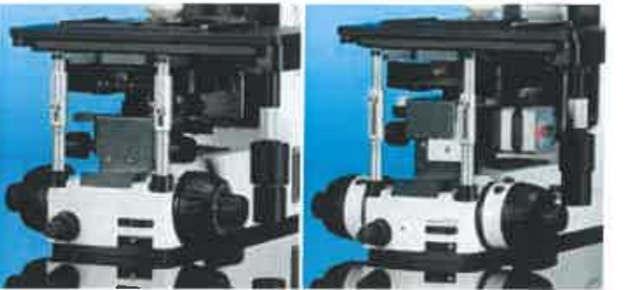
The control elements for focus drive, stage drive and condenser drive, for the selection of visible or infrared light, for adjusting the light field diaphragm, the regulation of light intensity and for all contrast techniques in transmitted-light are positioned at the very front of the stand. On the motorized stand (right) all the motors can be controlled with the keyrings.
