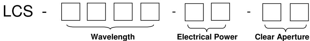
For example, LCE-0455-03-22 has a wavelength of 455nm, electrical power consumption of 3W, and a clear aperture diameter of 22mm.
