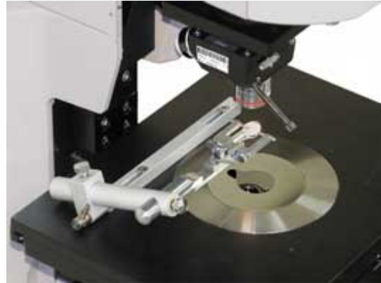
Example for Mounting on a microscope stage. Olympus BX51WI & Arm adjust adaptor.
