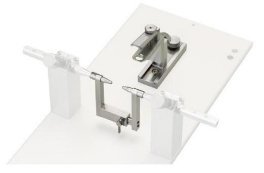
\* An ear bar for mice (<u>EB-3B</u>) can be attached to an auxiliary ear bar for rats (<u>EB-4N</u>).
