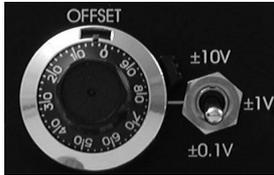
The OFFSET unit consists of (1) OFFSET range switch and (2) OFFSET potentiometer.
