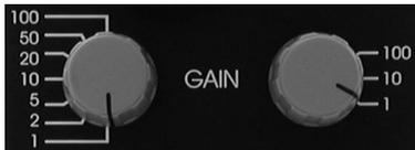
The GAIN unit consists of (3) GAIN range switch and (4) GAIN factors switch.
