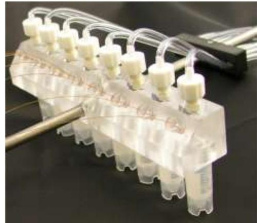
The tube needs to be gently pushed through the gasket. Apply a small amount of force to pierce the gasket, and then push the tube all the way down to the bottom of the reservoir, until the tube cannot go any farther.
