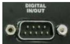
The digital input is used to control the valves via a TTL signal. The DB-9 male connector pins 1-8 is used to input TTL signals to valves 1-8, respectively, with pin 9 being common ground.
