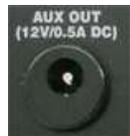
The AUX OUT port outputs 12V dc whenever any valve is turned ON. This port can be used to connect an additional 12V dc valve. Center pin on the connector is positive (+).
