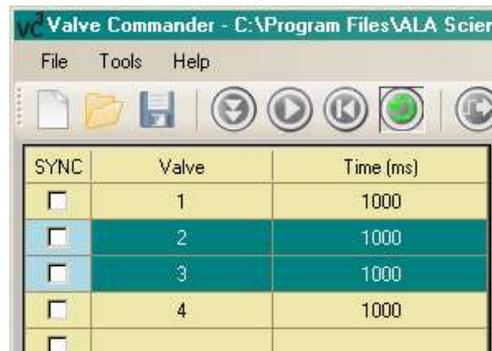
After inserting the loop, download the sequence to the VC<sup>3</sup> controller by pressing the download button.
