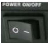
Power ON/OFF switch will turn the main power to the controller ON or OFF.
