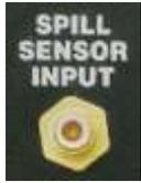
The VC<sup>3</sup> has been designed with a built in spill sensor. This feature will allow for the protection against overflows from chamber or dishes onto expensive optics or electronics.
