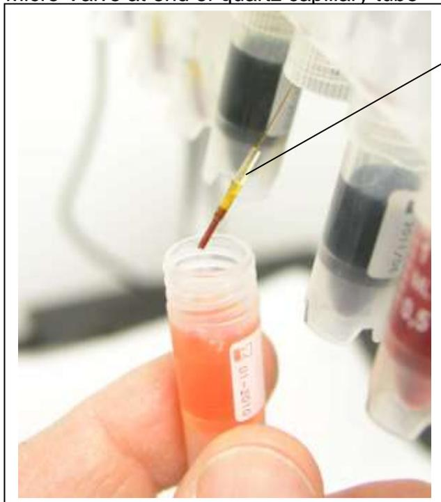
Insert the quartz capillary tube into the Silicone leader of the check valve. Do not push it past the Silicone tube leader.
