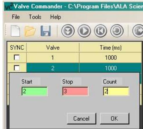
3. When a loop is inserted in the sequence the steps in the loop will be displayed as blue and dark green.
