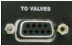
This DB-9 Female port is used to connect the controller to the valve manifold (VM-4/8).
