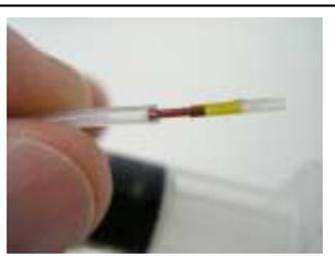
Remove the Micro valve from the quartz capillary, and using a syringe with a 1mm ID length of silicone tubing, inject water into the valve. About 1ml is all that is needed to flush out the valve. After flushing you can test the Micro valve by pulling back on the syringe. If the valve is working, the plunger will not remain extended after letting go.
