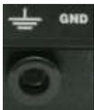
The VC<sup>3</sup> controller can be connected to ground via a banana jack on the rear panel.
