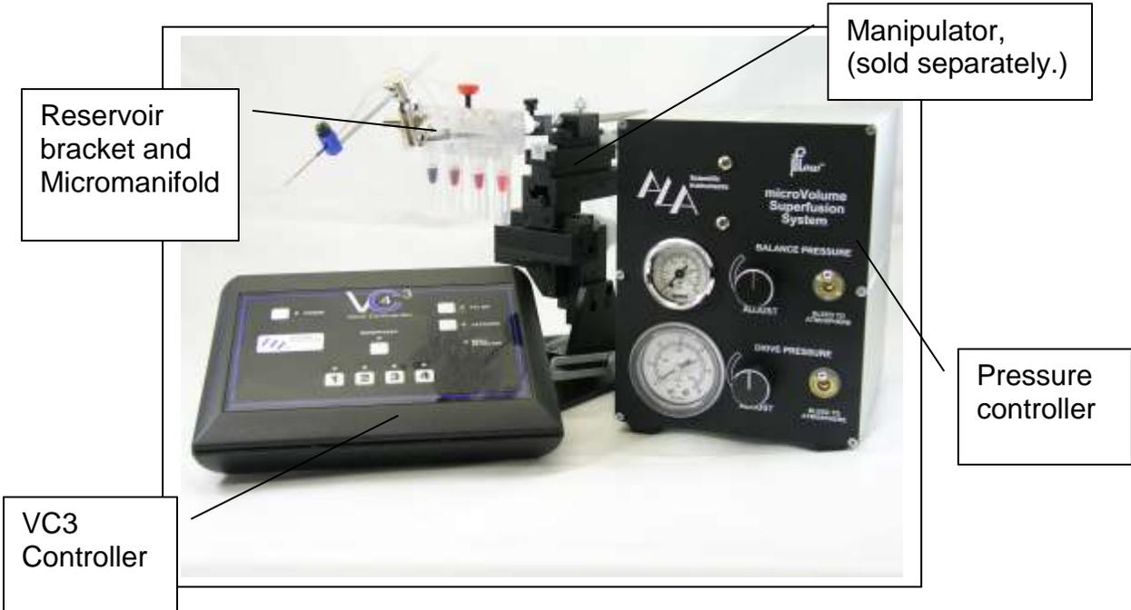
The reservoir bracket and Micromanifold must be mounted so that the Micromanifold can reach the prep, to minimize flow due to gravity mount the Micromanifold level with the reservoirs.
