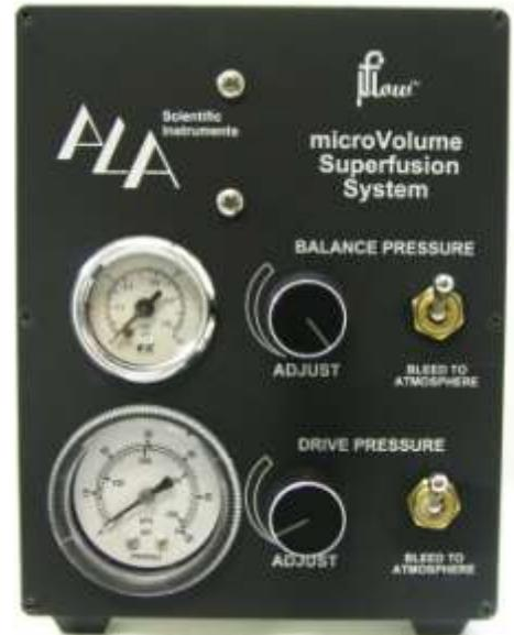
The **Low Pressure, "Balance Pressure"** on the front panel (up to 10psi (.690bar)) consists of an analog pressure gauge, a pressure regulator and bleed switch. The balance pressure is used to supply pressure to one reservoir (usually number 1) to provide a wash solution that keeps the other solutions at bay in their respective tubes. It can also be used in other ways in different configuration described later in this manual.
