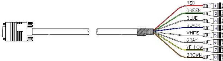
Cable is color coded according to above image. Red corresponds to valve1, green to valve 2 and so forth. Connect the DB-9Female connector to the rear of the VC<sup>3</sup> controller. Connect the BNC 's to the digital outputs of your acquisition system.
