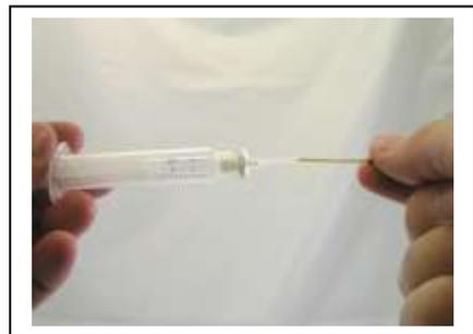
Micromanifolds® can be stored wet or dry. If calcium builds up internally, flush with vinegar for at least 1 hour and then distilled water. Micromanifolds can also be sonicated.
