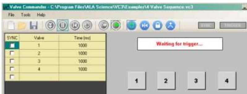
Send a TTL high signal to the Trigger IN port (Analog IN port) of the VC<sup>3</sup> controller to trigger the system to begin the sequence.
