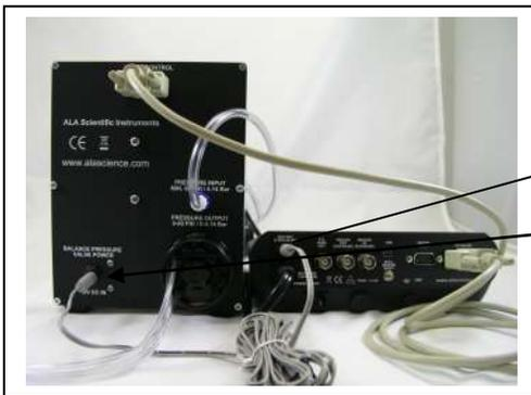
“Balance Pressure Valve” is plugged into 12 Volt Output on VC3 controller.
