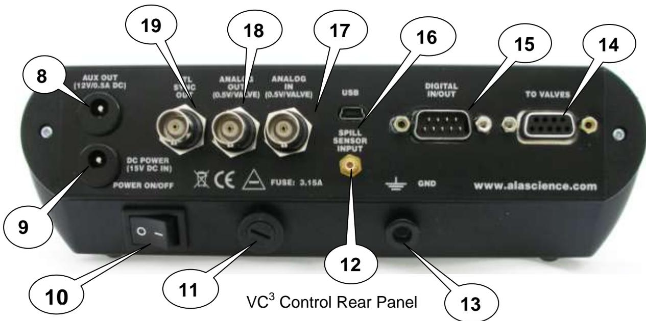
**8. AUX OUT 12V DC-** Port for additional 12V dc valve connection. Positive center pin.
