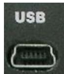
The USB connector is used to connect the VC<sup>3</sup> controller to a computer. This port is used for programming and maintenance at the factory only.
