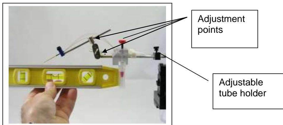
The manifold assembly comes mounted to a 6mm bar that can fit in most manipulators. The entire assembly in an 8 channel system will be about 150g, so be sure that the micromanipulator can handle it. Try to keep the assembly horizontal and move the parts around using the adjustment points shown above to keep the output tip at the same level as the fluids in the reservoirs.
